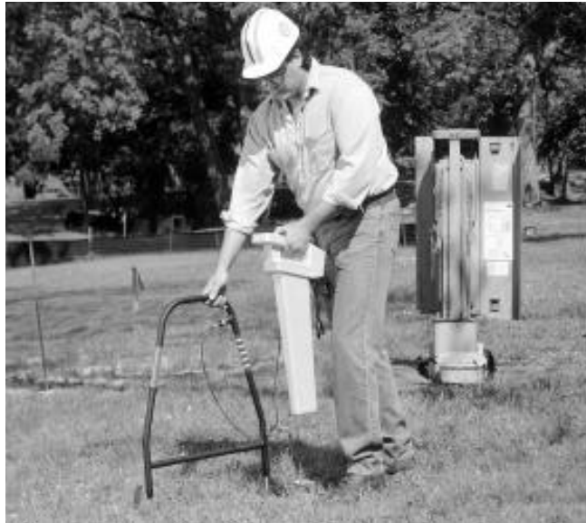
The Dynatel 2273E Cable/Fault Locator locates sheath (earth return) faults. 3
