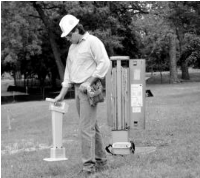
The Dynatel 2273E Cable/Fault Locator can be used with the Dynatel 2205/2206 EMS Marker Locating Accessory. 2
